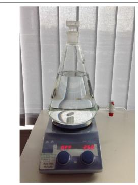
Fig. 1 Typical WAF test medium preparation set-up
