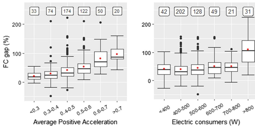
**Fig. 6** Relationship between FC gap and parameters related to  $a_{pos}$  as a proxy of driving style and power consumption (the box represents the 1st and 3rd quartile; line is the median FC; red dot is the mean, whiskers represent 1.5\*IQR (interquartile range), black dots are values below or higher than 1.5\*IQR, and numbers on top of the graphics are the number of segments in each selected bin)
