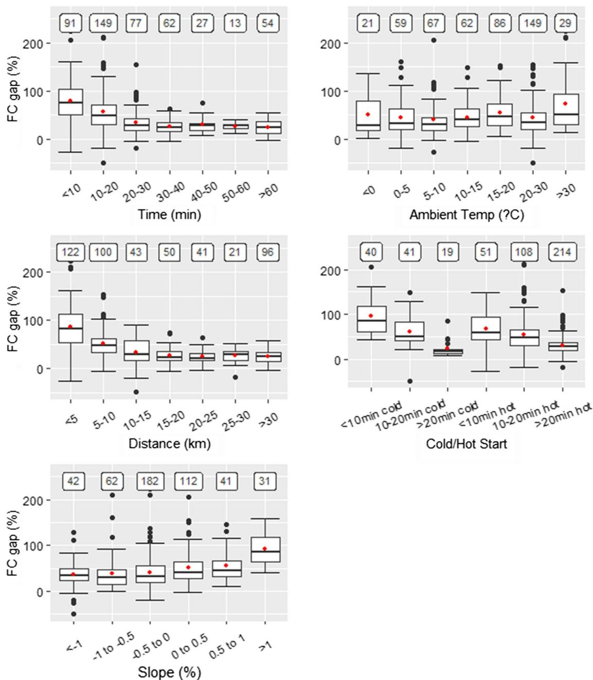
**Fig. 4** Relationship between FC gap and parameters related to trip characteristics (trip duration, distance, and road grade), ambient temperature and cold/hot start (the box represents the 1st and 3rd quartile; line is the median FC; red dot is the mean, whiskers represent 1.5\*IQR (interquartile range), black dots are values below or higher than 1.5\*IQR, and numbers on top of the graphics are the number of segments in each selected bin)
