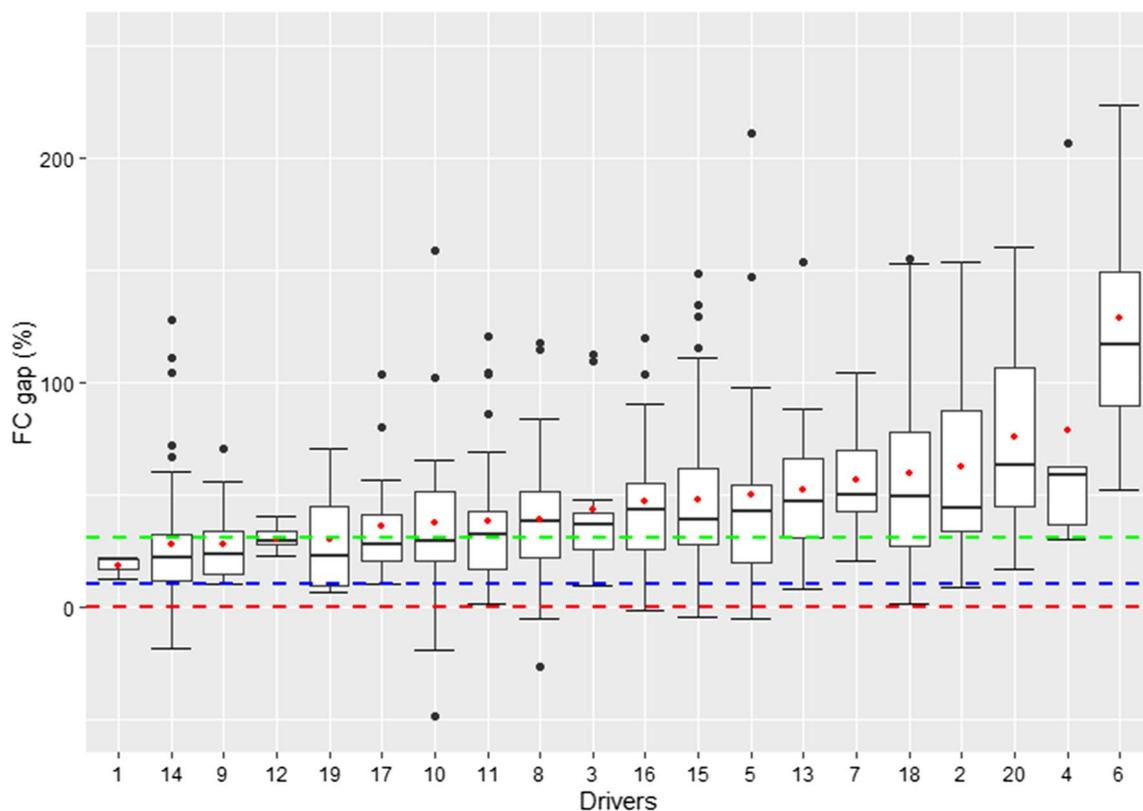
**Fig. 5** Variation in FC gap grouped by drivers and sorted by mean values (from lowest to highest value). The box represents the 1st and 3rd quartile; line is the median; red dot is the mean; whiskers represent 1.5\*IQR; and dots values below or higher than 1.5\*IQR (red dashed line represents the official NEDC-based FC gap (0%); blue dashed line represents the WLTP FC gap; and green dashed line represents the PEMS FC gap)
