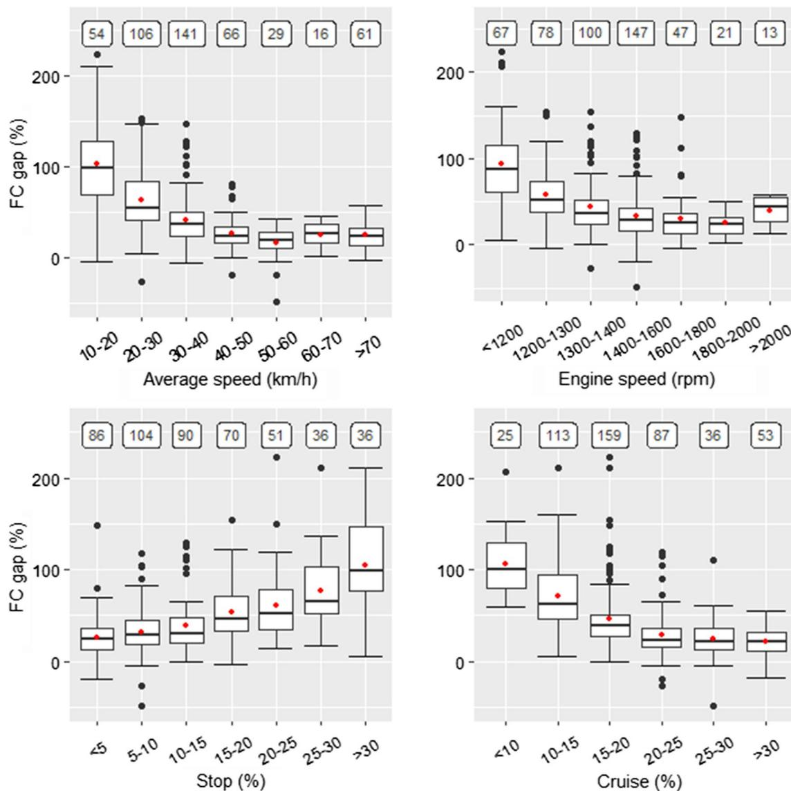
**Fig. 3** Relationship between FC gap and parameters related to traffic congestion (the box represents the 1st and 3rd quartile; line is the median FC; red dot is the mean, whiskers represent 1.5\*IQR (interquartile range), black dots are values below or higher than 1.5\*IQR, and numbers on top of the graphics are the number of segments in each selected bin)
