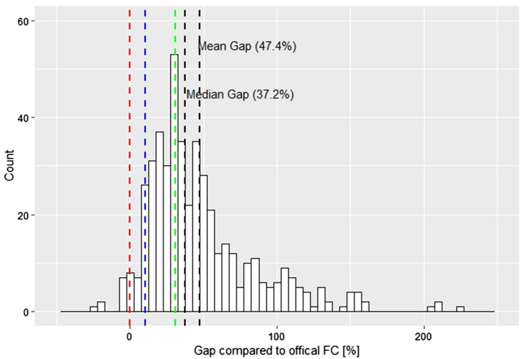
**Fig. 1** Histogram of the FC gap from all individual RWD trips (red dashed line represents the official NEDC-based FC gap (0%); blue dashed line represents the average WLTP FC gap; and green dashed line represents the average PEMS FC gap)
