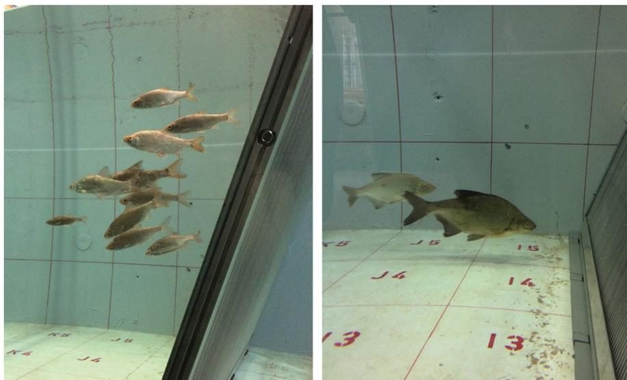
**Fig. 4** Behavioural studies on fish within the flow channel. Different types of bar racks are tested on common roaches (*Rutilus rutilus*, left) and common breams (*Abramis brama*, right)
