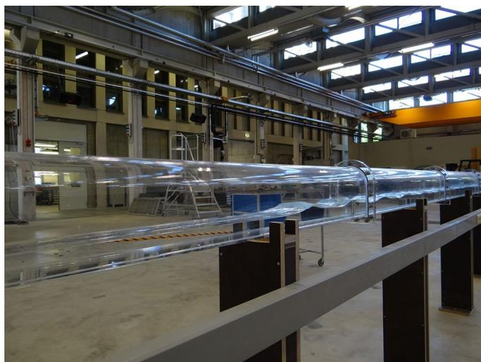
**Fig. 5** Model of underground pumped-storage plant. With a length of about 36 m, the model is used to assess flow conditions in cavities
