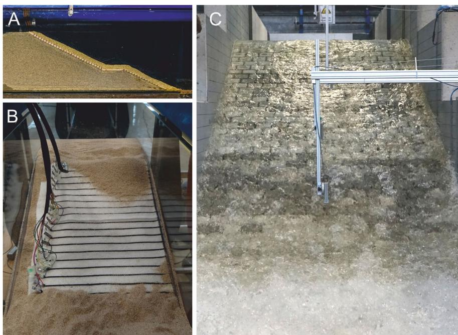
**Fig. 6** Dike models used in project EarlyDike. **A** Small-scale model, equipped with intelligent geotextile **(B)** for detection of water; **C** overflow of large-scale dike model
