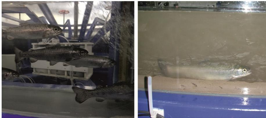
**Fig. 3** Hydro-toxic studies on sediment-bound pollutants in the circular flume at IWW. Rainbow trouts (*Oncorhynchus mykiss*) were exposed to clear water (negative control, left) and water-sediment-mixtures (right) that were artificially spiked with environmental pollutants, e.g., polycyclic aromatic hydrocarbons
