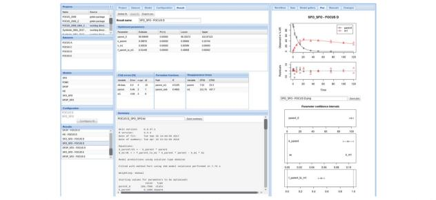
**Fig. 4** Screenshot of gmkin 0.6.7 Datasets and models are listed on the left, numerical results and a summary are shown in the center and a plot of the fitted model is on the right
