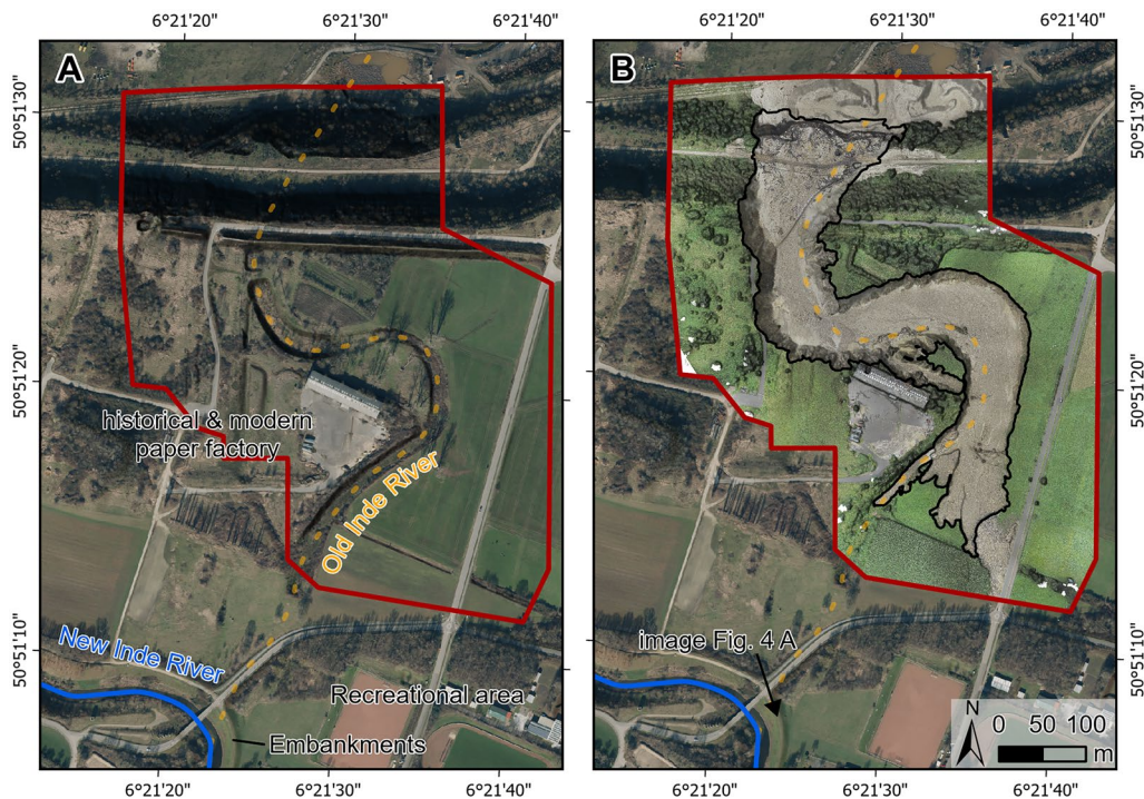
Fig. 2 Changes in the relief of the study area before (A) and after (B) the 2021 flood event, when the Inde River had entered the open-cast mine. Symbology is adapted from Fig. 1
