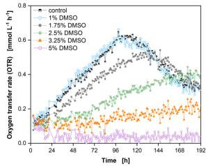
**Fig. 5** Influence of DMSO on the oxygen transfer rate (OTR) of CHO cell line two. The OTR over time is depicted in the presence of 0% DMSO (= control) (black squares), 1% DMSO (open blue diamonds), 1.75% DMSO (closed gray circles), 2.5% DMSO (open green stars), 3.25% DMSO (closed orange triangles), or 5% DMSO (open purple circles). DMSO was added at the beginning of the cultivation (t = 0 h). Data from experiment 6 (Additional file 1: Table S1)
