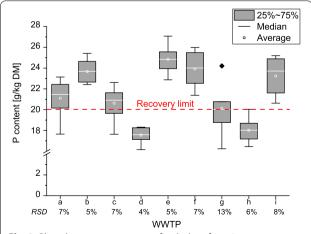
**Fig. 2** Phosphorus content ranges for sludges from 9 wastewater treatment plants (WWTPs). Relative standard variations below
