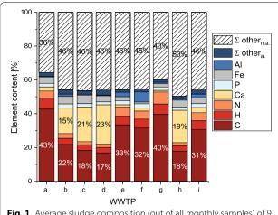
**Fig. 1** Average sludge composition (out of all monthly samples) of 9 wastewater treatment plants (WWTPs)
