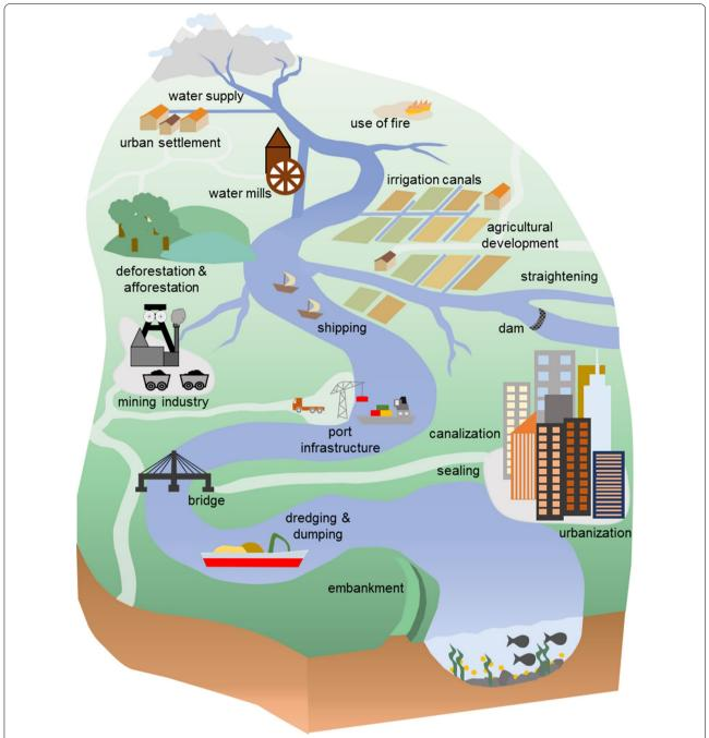
Fig. 1 Schematic diagram of human impact factors on river–floodplain systems in Western Europe since the beginning of the Holocene (modified after [33] already published in [57])
