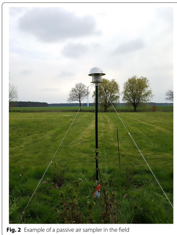
**Fig. 2** Example of a passive air sampler in the field
