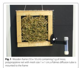
(driving force) along the length of the tube.  $NO_2$  diffusion tubes were located next to the moss-samplers, both indoor and outdoor (see Fig. 1). Each tube was exposed for 1 month and then replaced by a new tube deployed during the second month.
