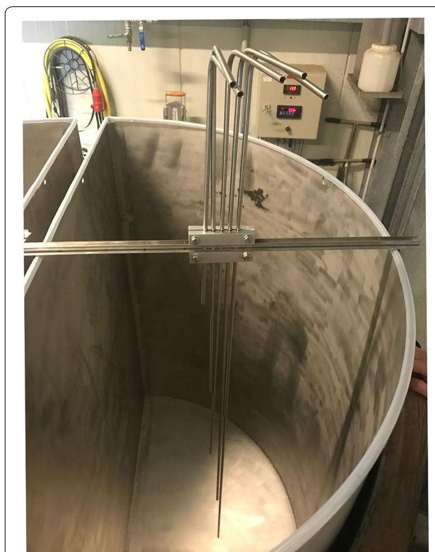
Fig. 1 Steel tubes for water sampling at different depths without disturbing the water body
