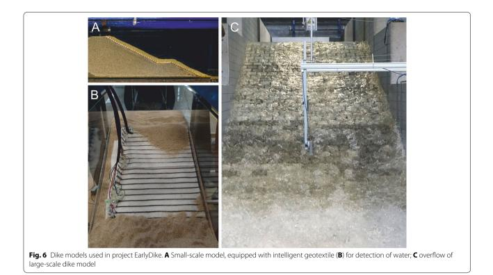
real-time and allow for quick protective and action measures in case of an impending dike failure [9]. The studies at IWW are supported by numerical analysis and aim to develop a flooding simulation software to predict flooding-affected areas, resulting consequences and mechanical durability of protective structures.
