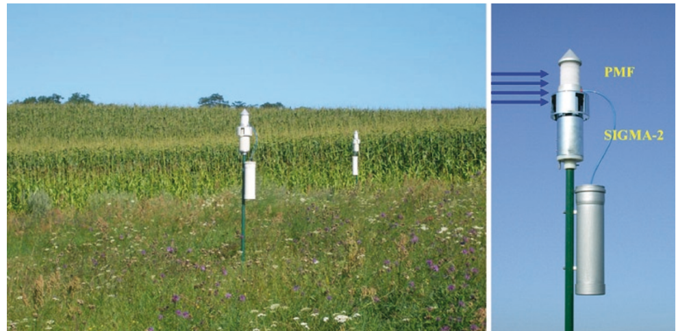
Fig. 2 Technical pollen sampler PMF/Sigma-2. Left: Site I, measuring points #1a at 5 m distance and #2 at 26 m distance to maize field edge (4 August 2007) (Picture: Hofmann)
