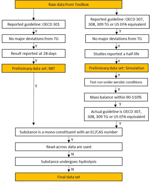
Fig. 1 Process for screening RBT and simulation test data
